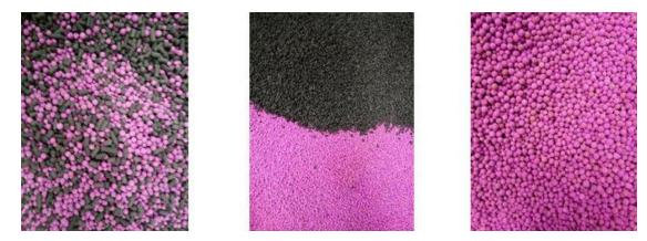
Activated carbon media can be used for the remediation of vapors generated, the removal of VOCs from the air, soil venting and removal of other organics such as ammonia, sulfur compounds, mercury, and amines.
