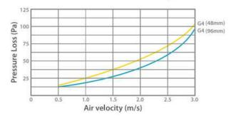
**Pro-Clean POLY-PLEAT** filters are cleanable / washable panel filters made up of non woven, high lofted synthetic (polyester) filter media and are available in various efficiency grades ranging from G2 to F5. POLY PLEAT filters offer very high dust holding capacity combined with lower resistance than the other types of similar grade panel filters.
