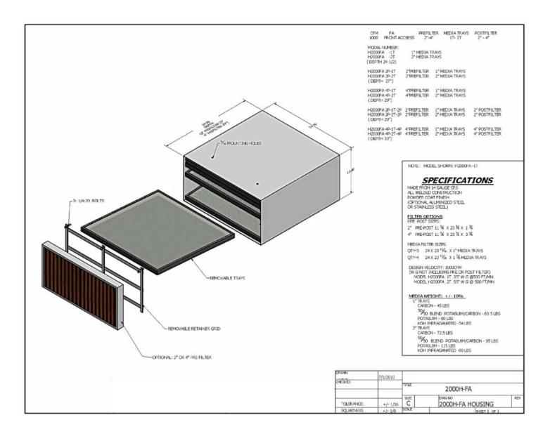
Front or Rear load Box style housing ½ size for 1"or 1.88" thick carbon trays 24" depth
