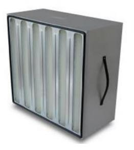
4V operates at very high air velocity up to 2000 CFM if required delivering a very low pressure drop. The V shaped arrangement allows more air flow per filter wherein a standard filter replacement can save up to 30% energy savings. Filters are light weight and its fully plastic body makes it incinerable as well.
