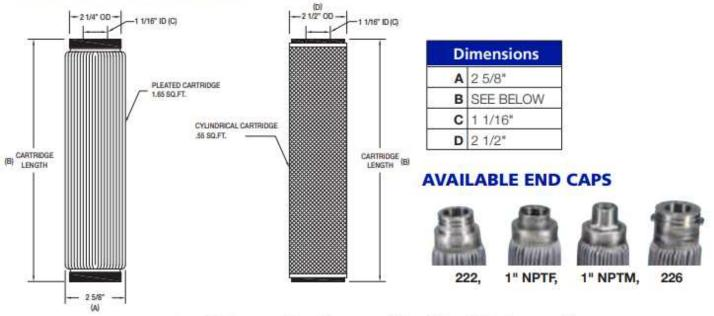
recommends not to flow more than 10 gpm per 10" cartridge at 40 microns and lower.
