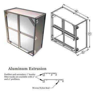
**V** Bank filter housing is a permanent single stage unit designed to hold pleated ASHRAE rated filters. The unit can accommodate both 2" and 4" filters in a low-pressure drop configuration. The V Bank unit is manufactured out of either galvanized steel or optional stainless steel and is welded and or bolted together. Each housing is custom manufactured to meet specific end user requirements
