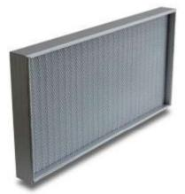
HT pleat filters are designed as a pre filter operating at high temperatures up to 500°F/260° C, with low pressure drop and long service life. Filters are classified with MERV8/G4/EU4 efficiency. They are made with a pleat distribution of 13 pleats per linear foot and are recommended to operate up to 2000 CFM. These filters are available in 45mm (2") and 95mm (4") depths. Filter face area can be custom made in many dimensions and the maximum recommended pressure drop is 1.2"w.g./300 Pa.
