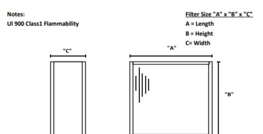
\*\*Glass media HEPA filters can flow either direction. The direction of airflow noted on filter is the direction the filter was tested before leaving the factory.
