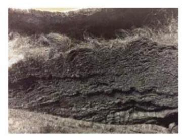
This image shows the outer part of the bag filter. It still has white areas. The outer bag is a support layer for the internal melt blown filter cartridge and is not expected to be full of contaminate, which happens with low efficiency filter bags
