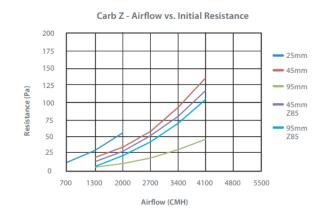
Rated face velocity is 1.5 m/s for 25mm and 2.5 m/s for 45 and 95mm
