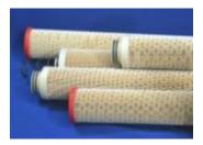
Elements offer economical, high quality Beta rated filtration for applications where "absolute" filters are required. Elements are available in cellulose, glass-cellulose and microglass media with a variety of end configurations and sizes. The pleated design ensures high contaminant retention due to the large surface area. Elements are available in ratings from 2 to 30 microns.
