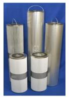
Designed for filtration of water, water based fluids, and a wide range of chemicals. These filter cartridges stand up to continuous use in water based fluids without the softening and/or deterioration common with many resin impregnated paper cartridges. These elements are made with an advanced synthetic polyester media, which allows high flow rates with low pressure drops as well as excellent temperature resistance.
